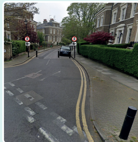
2 Alwyne Road Camera enforced traffic filter with bollards to narrow roadway, allowing emergency vehicles through. Two parking bays suspended.
