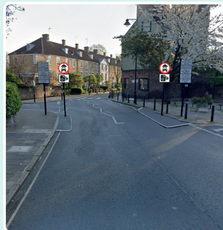
1 Canonbury Place Camera enforced traffic filter with kerb build outs to narrow roadway, allowing emergency vehicles through.
