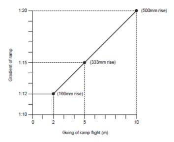
In no circumstances should the gradient exceed 1:12 and, where the overall level change is 2m or more, a lift should be provided instead.
