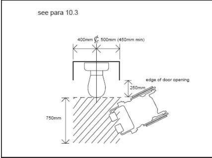
In all single storey dwellings and any dwelling with 3 bedrooms or more the entrance level WC should be wheelchair accessible. The wheelchair user must be able to close the door from within the closet. An outward opening door will normally be required. There should be a minimum of 700mm between the WC pan side rim and one sidewall, and 1100mm between the WC pan front rim and the opposite wall or door as illustrated on the Lifetime Homes website.
