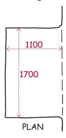
5.29 All halls and corridors (facilitating 90° turns) should have a clear unobstructed width of at least 1200mm and internal doors clear opening widths of at least 800mm. To facilitate a 180° turn a corridor width of 1500mm is required. The minimum pinch point admissible is 900mm. (Habinteg Guide pp57)
