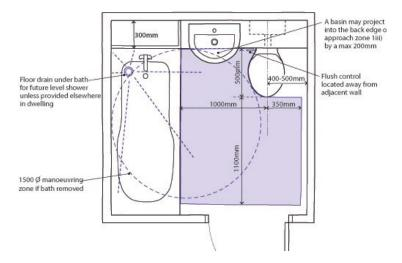
The bathroom should be designed for ease of access to the bath (or shower) WC and washbasin. This will normally require an outward opening door, and 1100mm between the front rim of the WC pan and the opposite wall.
