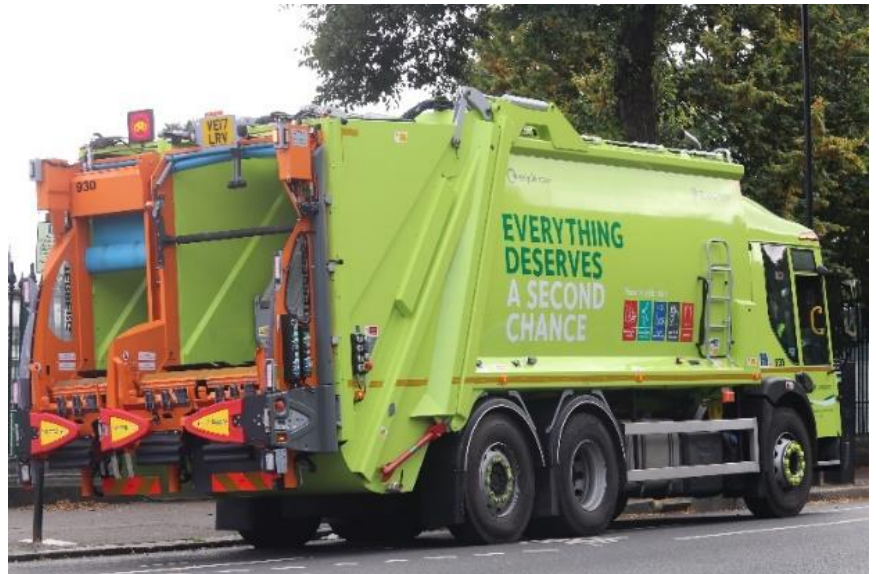
Figure 7 Split body vehicles collect recycling and organics in one vehicle to improve efficiency
