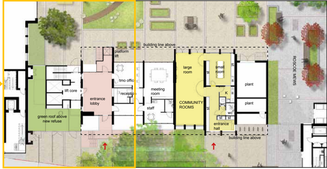
Upper Ground Floor Plan view of new community rooms; Braithwaite House entrance lobby and forecourt
