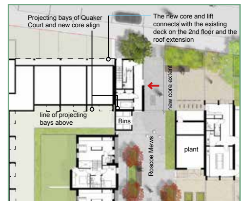
New Core 'C' with a lift at the end of QC terrace
