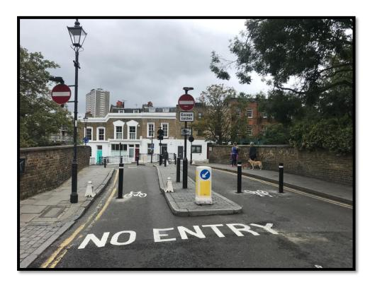
The filter on Danbury Street stops through-traffic from using Danbury Street as a short cut between Essex Road/Upper Street, New North Road and City Road. This filter uses bollards to stop people driving through.
