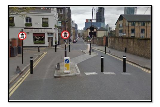
The filter on Wharf Road stops through-traffic from using St Peter's Street as a cutthrough between Essex Road/Upper Street and City Road. This filter uses bollards to stop people driving through and has removable bollards to allow emergency services through.
