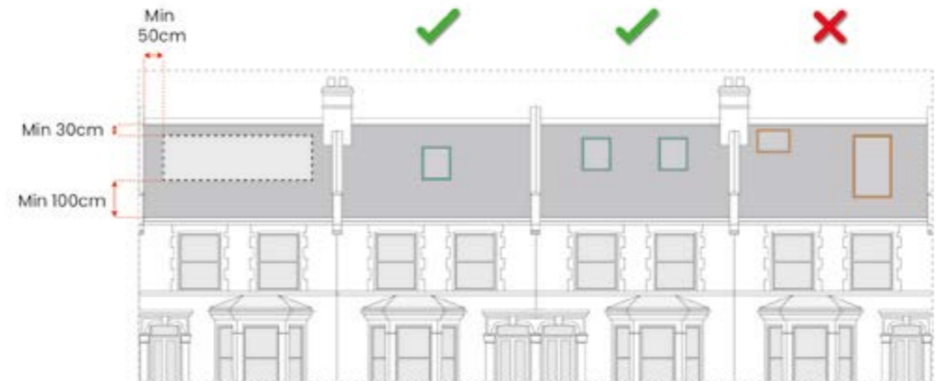
Image 29. Placement of rooflights on front roof slopes
